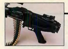
SS-77's left-folding buttstock is injection-molded over two steel pins which are integral with the investment-cast hinge mechanism. Note the thick recoil pad which reduces perceived recoil to an almost unnoticeable level. Photo: courtesy Lyttelton **Engineering Works**
